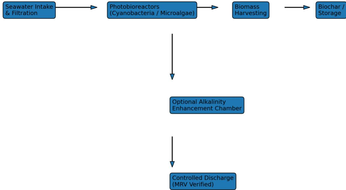
The diagram illustrates the controlled seawater intake, closed photobioreactor operation, biomass harvesting and sequestration pathway, optional alkalinity enhancement chamber, and monitored discharge under MRV protocols.
